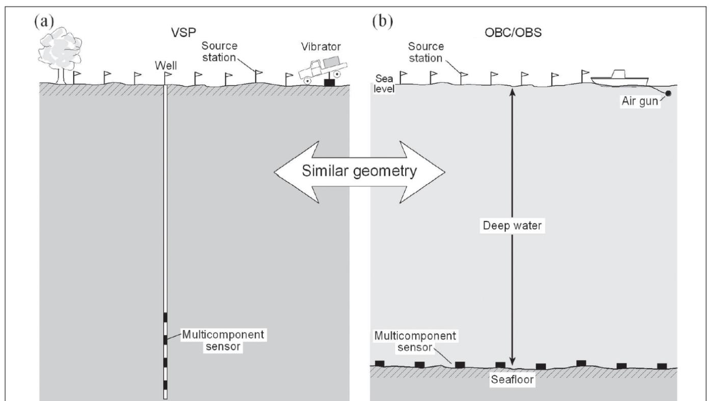
Figure 2 – Illustration of similar source-receiver geometries used for acquiring (a) VSP data and (b) deepwater OBC/OBS seismic data.
