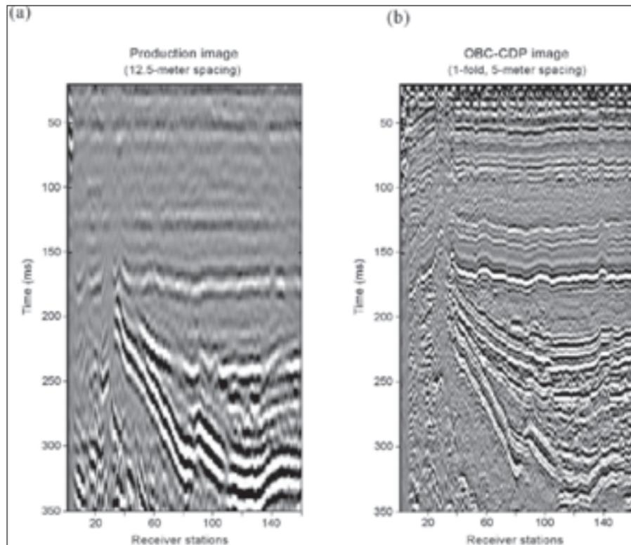
Figure 1(a) – Standard production processing of deepwater 4-C OBC seismic data along a profile that traverses a sea-floor gas-expulsion chimney. 1(b) Improved resolution of near-sea-floor geology using VSP-style concepts for processing deepwater OBC data. Both images are flattened to the sea-floor.
