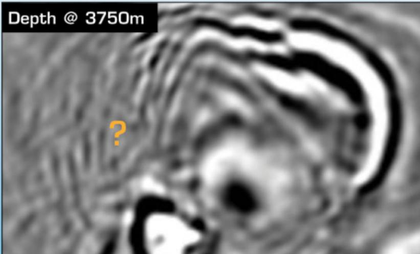
Sediment flood depth slice. Note the "hidden" TOS at the rim of the mini basin.
