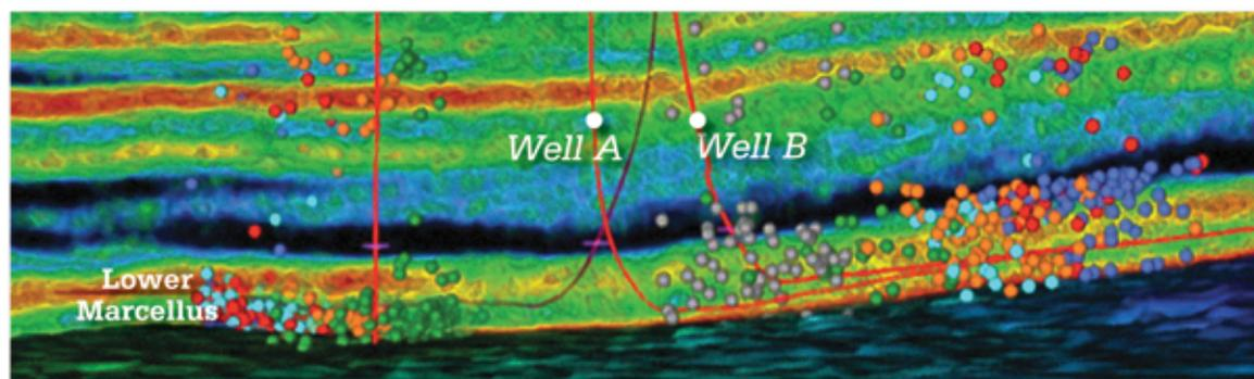
*Thickness of the ductile layer above the Lower Marcellus (blue) influences the degree to which fracs remain constrained.*
