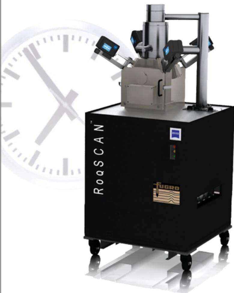
RoqSCAN™, the world's first ruggedized Scanning Electron Microscope based platform dedicated for wellsite applications, developed exclusively by Fugro and Carl Zeiss.
