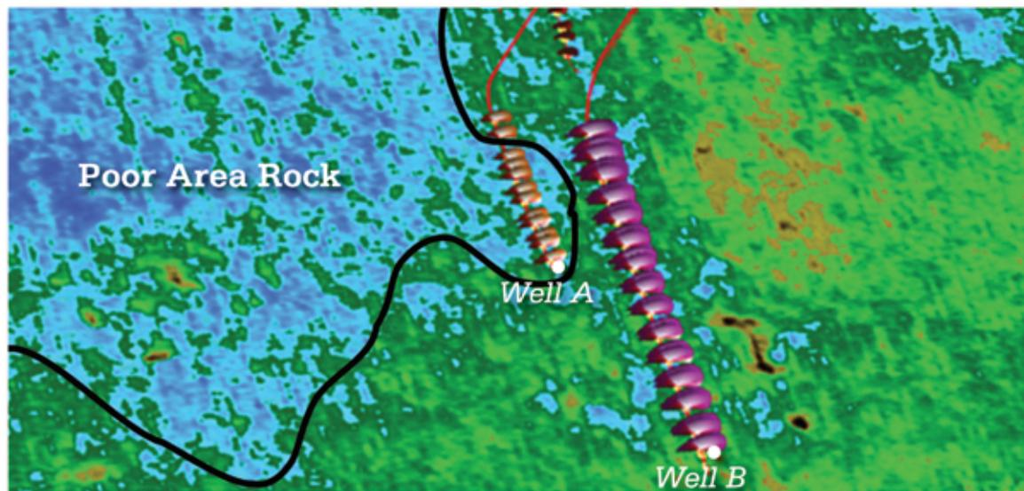
*Here, results show that stimulation programs can be optimized based on rock properties from seismic. Elimination of one frac stage per well can deliver a dramatic return on investment. Well B yielded twice the “production per foot” compared to Well A in this survey.*
