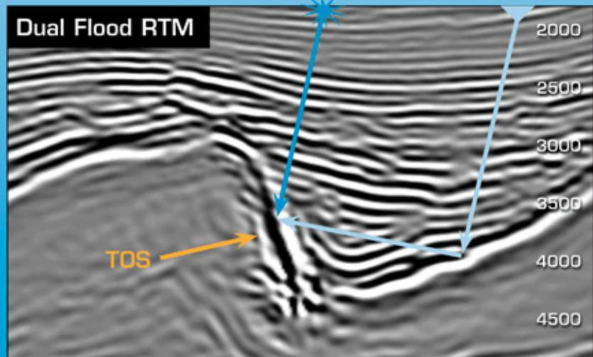
Same crossline after Dual Flood RTM. Better imaging results in more accurate interpretation of the salt geometry.
