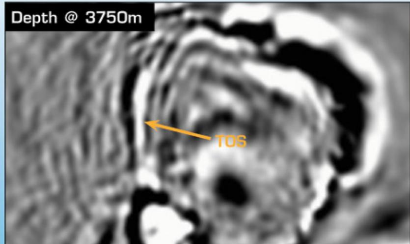
Same depth slice after Dual Flood RTM. Prism waves image the salt flank, giving an accurate geometry to the mini basin.
